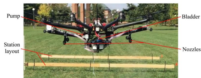
Figure 1 Aerial spray system based on a DJI S1000 octocopter
