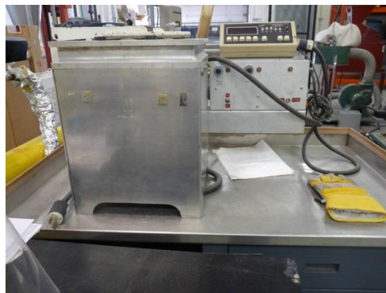
Figure 2 The tangential abrasive dehulling device
