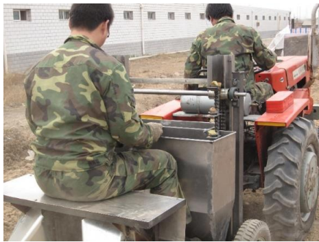
Notes: The potato planter must be equipped with a special station behind it to facilitate manual compensation for miss-seeding.
