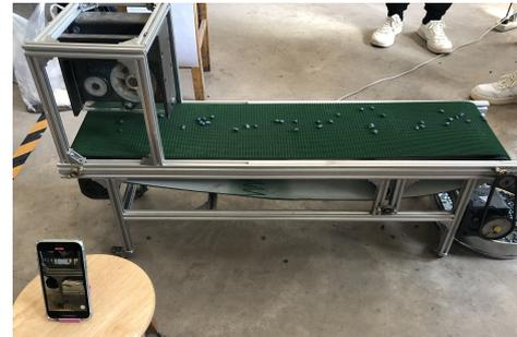
Figure 16 Metering seed device
