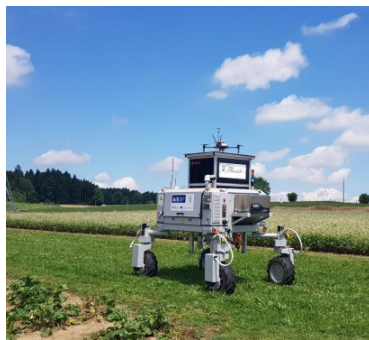
Figure 2 Unmanned ground vehicle Bonirob, carrying an unmanned aerial vehicle [27]
