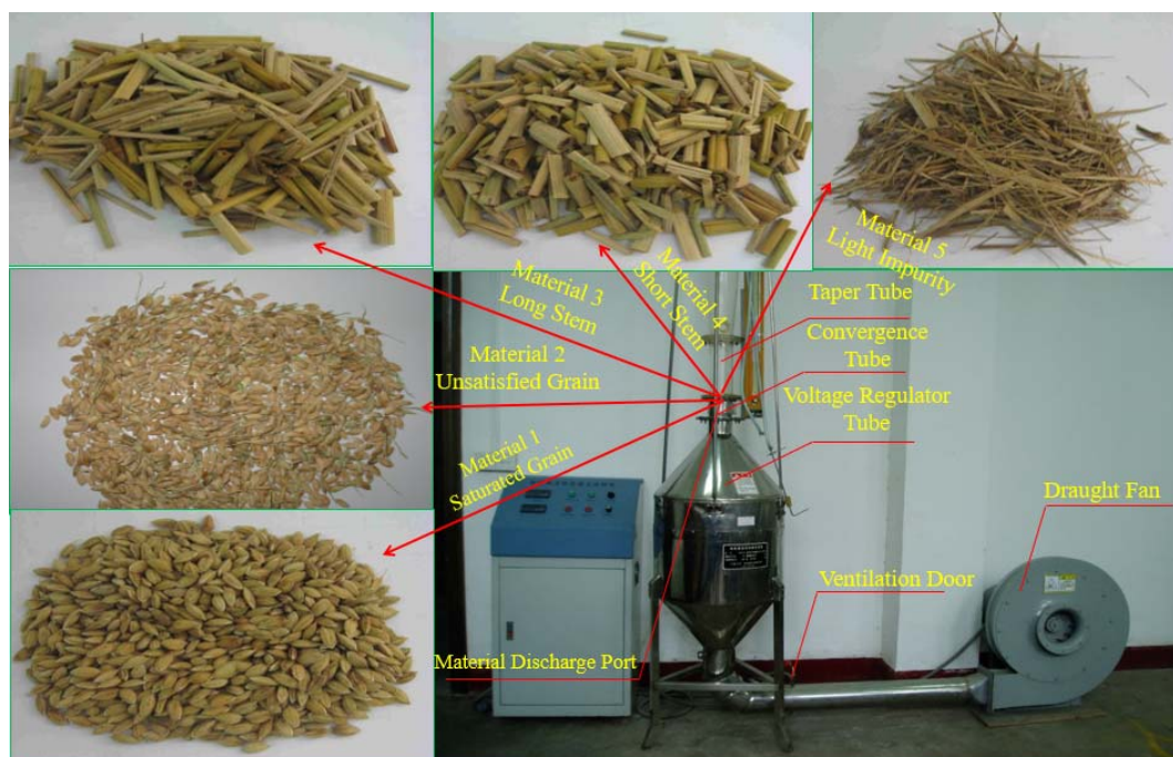
Figure 1 DFPF-25 material floatation-specific measuring device and material
