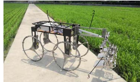
1. Paddy walking platform 2. Connecting mechanism 3. Weeding equipment
