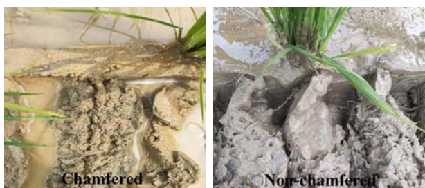
Figure 10 Weeding effects of chamfered and non-chamfered weeding roller
