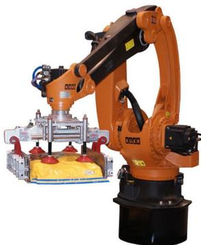
b. Kuka Palletizing robot KR 40 PA
