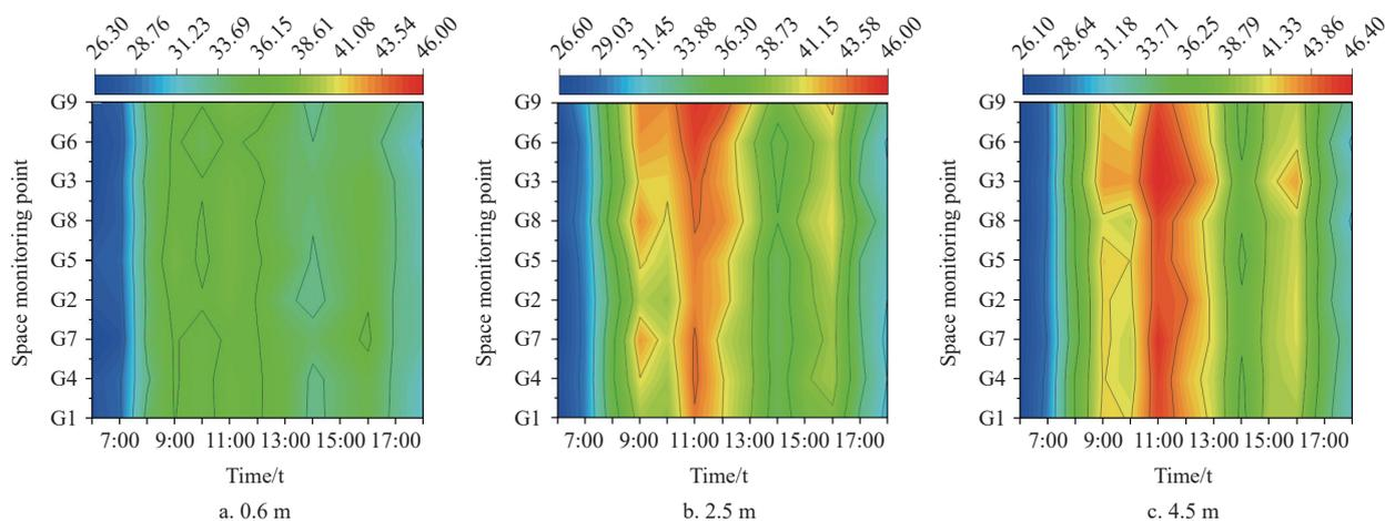
Figure 3 Contour cloud map of different monitoring plane temperatures in the greenhouse
