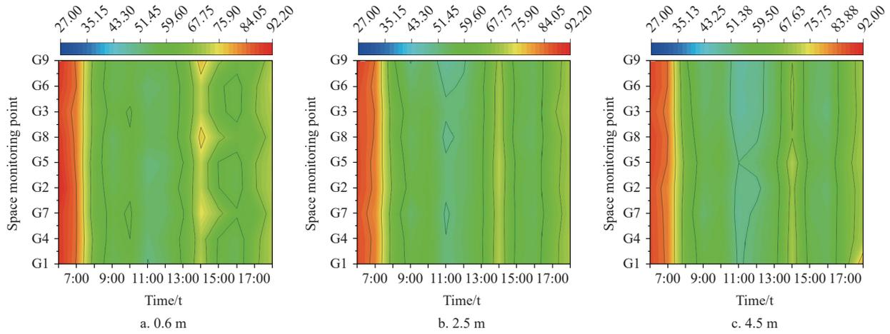
Figure 5 Humidity changes at different monitoring heights in the greenhouse
