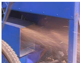
b. Discharge process of short stems, glumes and light impurities
