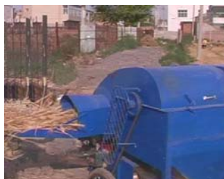
a. Threshing and cleaning device for plot-bred wheat
