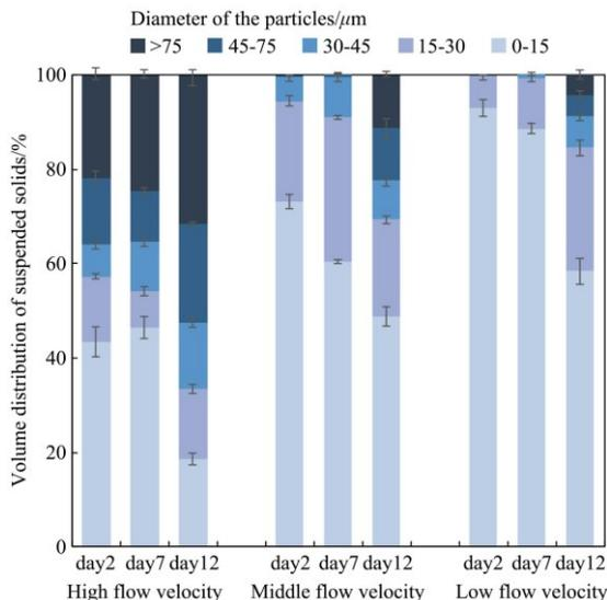
Figure 4 Volume distribution of suspended solids in RAS
