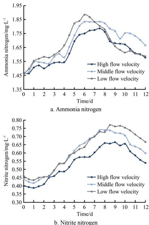
Figure 2 Changes of ammonia nitrogen and nitrite nitrogen within 12 h after feeding under different flow velocities
