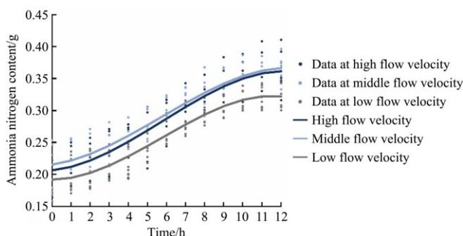
Figure 7 Ammonia nitrogen content model at different flow velocities
