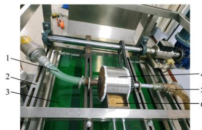
1. Positive pressure air supply pipe 2. Seed metering device holder 3. Seed bed belt 4. Roller 5. Negative pressure air supply pipe 6. Seed box
