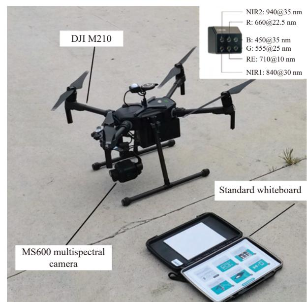
Figure 1 DJI M210 and MS600 multispectral camera
