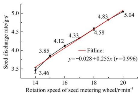
Figure 10 Seed discharge rate under different rotation speeds of seed metering wheel
