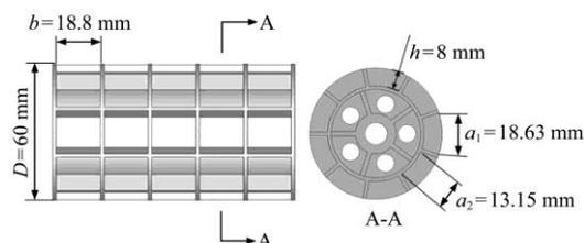
Note:  $D$  is the diameter of seed metering wheel, mm;  $b$  is the width of seed metering wheel chamber, mm;  $h$  is the depth of seed metering wheel chamber, mm;  $a_1$  is the top length of seed metering wheel chamber, mm;  $a_2$  is the bottom length of seed metering wheel chamber, mm
