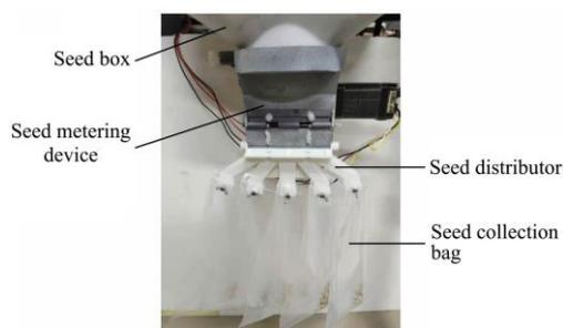
Figure 5 Seed metering device test
