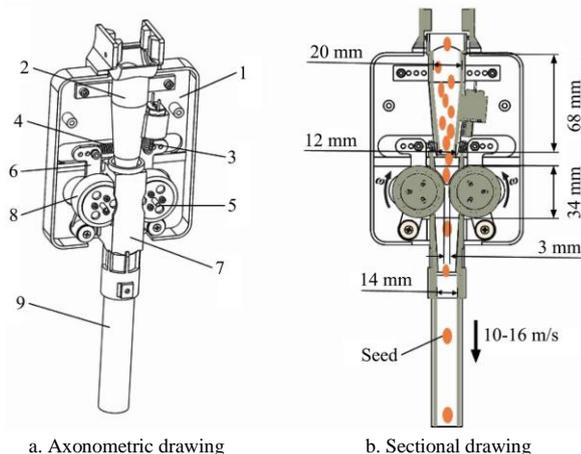
a. Axonometric drawing b. Sectional drawing
