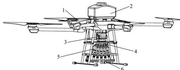
1. UAV platform 2. Seed box 3. Seed-metering device 4. Seed distributor
