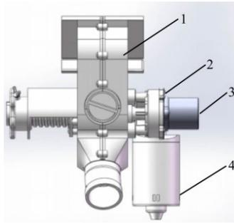
1. External groove wheel type fertilizer apparatus 2. Deceleration gear
