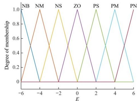
Figure 5 Affiliation function curve of the input variable
