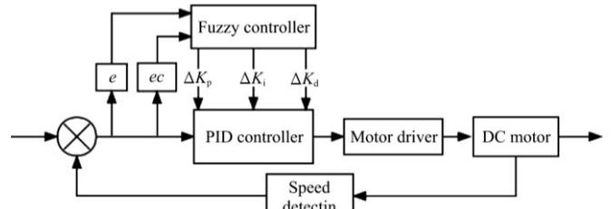
Figure 4 Fuzzy PID control block diagram
