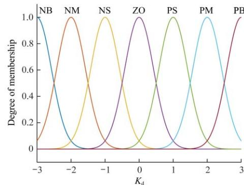
Figure 6 Affiliation function curve of the output variable
