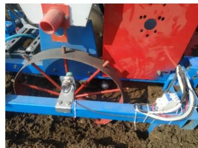
Figure 2 Schematic diagram of ground wheel speed detection
