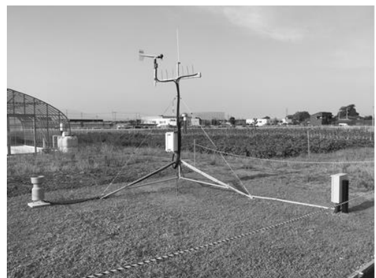
Figure 13 A weather station in the field smart farm (A data logger is connected with PC via LAN)
