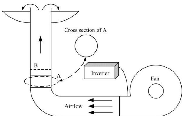
Figure 1 A schematic diagram of the terminal velocity analyzer
