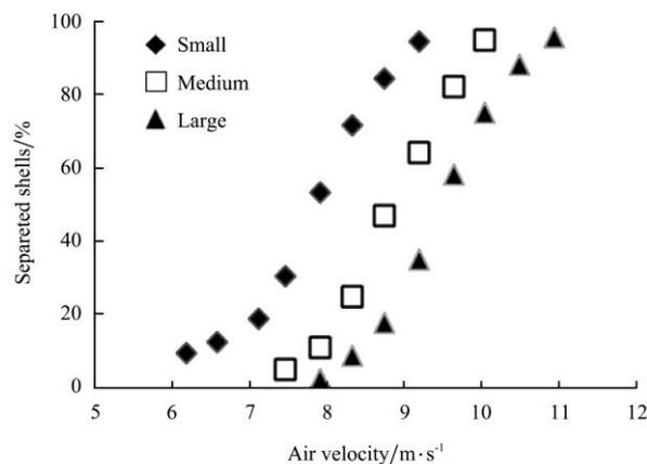
Figure 2 Separation of the walnut shells at different air velocities for three particle sizes of small, medium and large for the variety of Poost-Sangi
