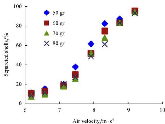
Figure 3 Separation of the walnut shells at different air velocities for four feeding values of 50, 60, 70 and 80 g for the variety of Poost-Sangi
