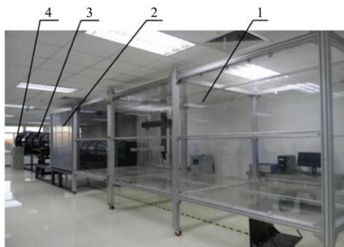
1. Test section 2. Steady section 3. Contraction section 4. Centrifugal blower
