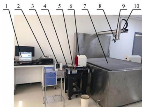
1. Computer 2. Mechanical arm controller 3. Power supply 4. PWM controller 5. Solenoid valve 6. Laser particle size analyzer 7. Droplet collection device 8. Pressure gauge 9. Nozzle 10. Motor driving two-dimensional arm
