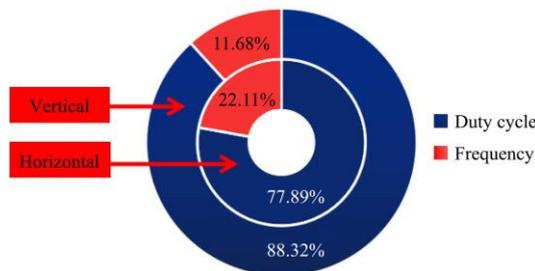
Figure 8 Influence weights of the PWM duty cycle and frequency on spray drift
