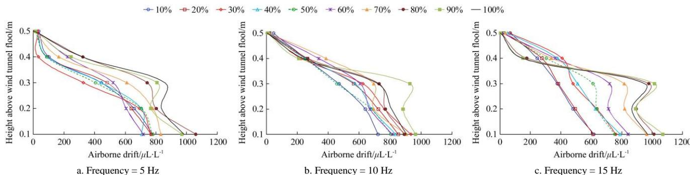
**Figure 6 Airborne drift curves in the vertical profile under various PWM working conditions**
