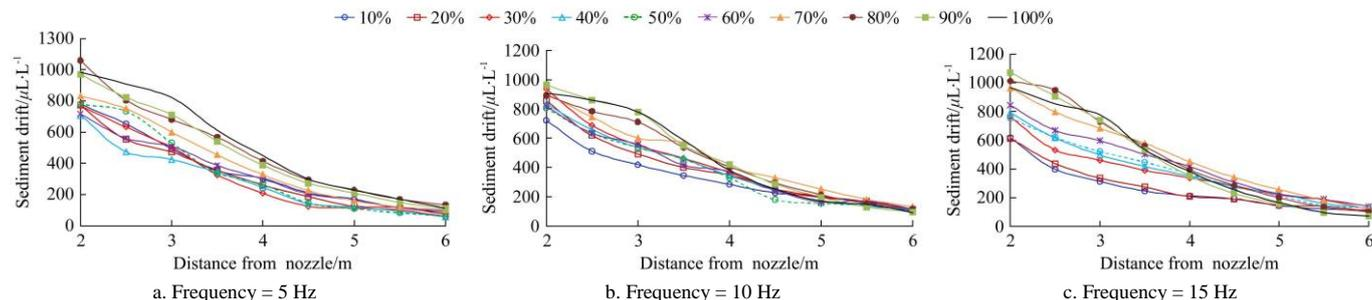
**Figure 7 Sediment drift curves in the horizontal plane under various PWM working conditions**
