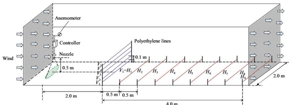
Figure 4 Schematic layout of the collecting line arrangement in the wind tunnel
