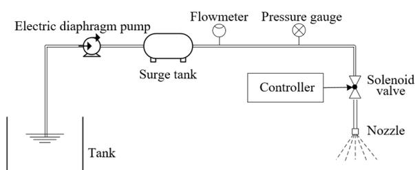
Figure 1 PWM variable-rate spraying system
