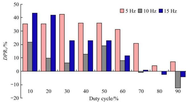
Figure 9  $DP_{R_V}$  for different PWM frequencies and duty cycles
