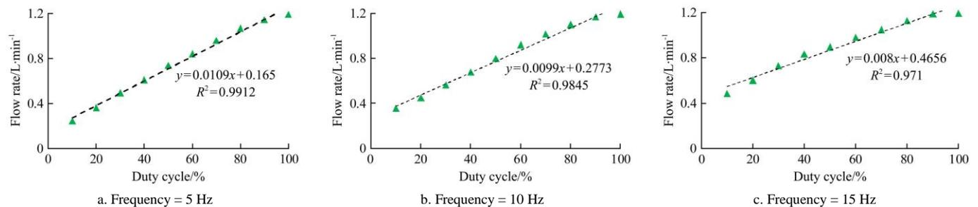
Figure 5 Nozzle flow rates with different PWM frequencies and duty cycles
