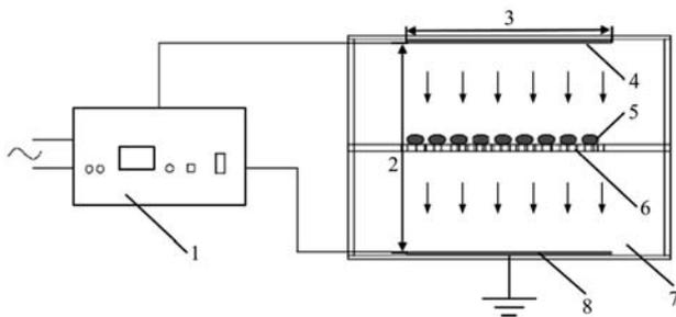
1. LFHV-PEF generator 2. Copper plate spacing 3. Copper plate size
