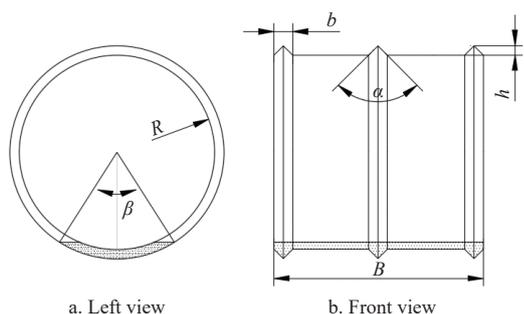
Note:  $R$  is the radius of the soil-covering and soil-compacting wheel, cm;  $\beta$  is the subsidence angle, ( $^\circ$ );  $\alpha$  Sharp angle, ( $^\circ$ );  $h$  is the height of sharp angle, cm;  $b$  is the width of sharp angle, cm;  $B$  is the length of the soil-covering and soil-compacting wheel, cm.
