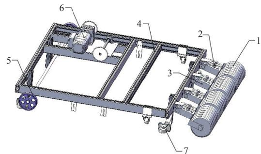
1. Soil-covering and soil-compacting wheel 2. Ballast pressure regulator 3. Fixing frame of soil-covering and soil-compacting wheel 4. Rack 5. Traveling wheel 6. Motor 7. Limit wheel
