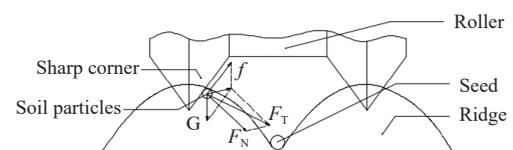
Note:  $G$  is the self weight of soil particles,  $N$ ;  $F_N$  is the supporting force of soil particles by the soil-covering and soil-compacting wheel,  $N$ ;  $f$  is the friction force of soil particles subjected to the soil-covering and soil-compacting wheel,  $N$ ;  $F_T$  is the synthetic force of each force,  $N$ .
