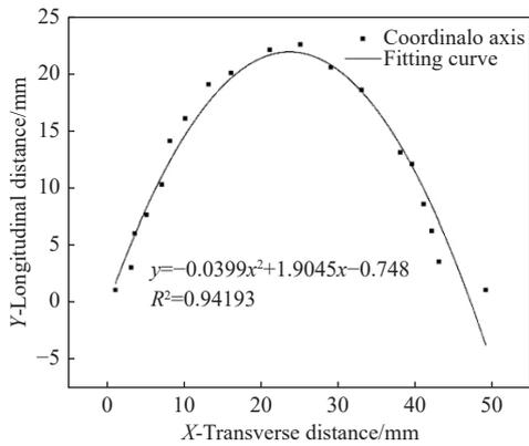
Figure 3 Curve fitting of seed furrow contour (ridge)
