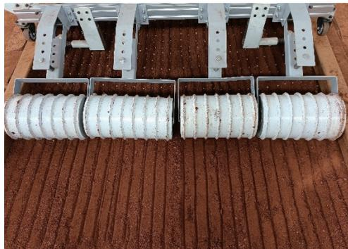
Figure 13 Soil-covering and soil-compacting process
