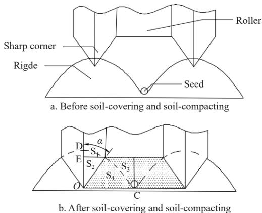
Figure 4 Schematic diagram of seeds and soil after soil-covering and soil-compacting
