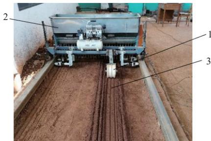
1. Soil-covering and soil-compacting wheel 2. Panax notoginseng seedling seeding precision planter 3. Soil trough
