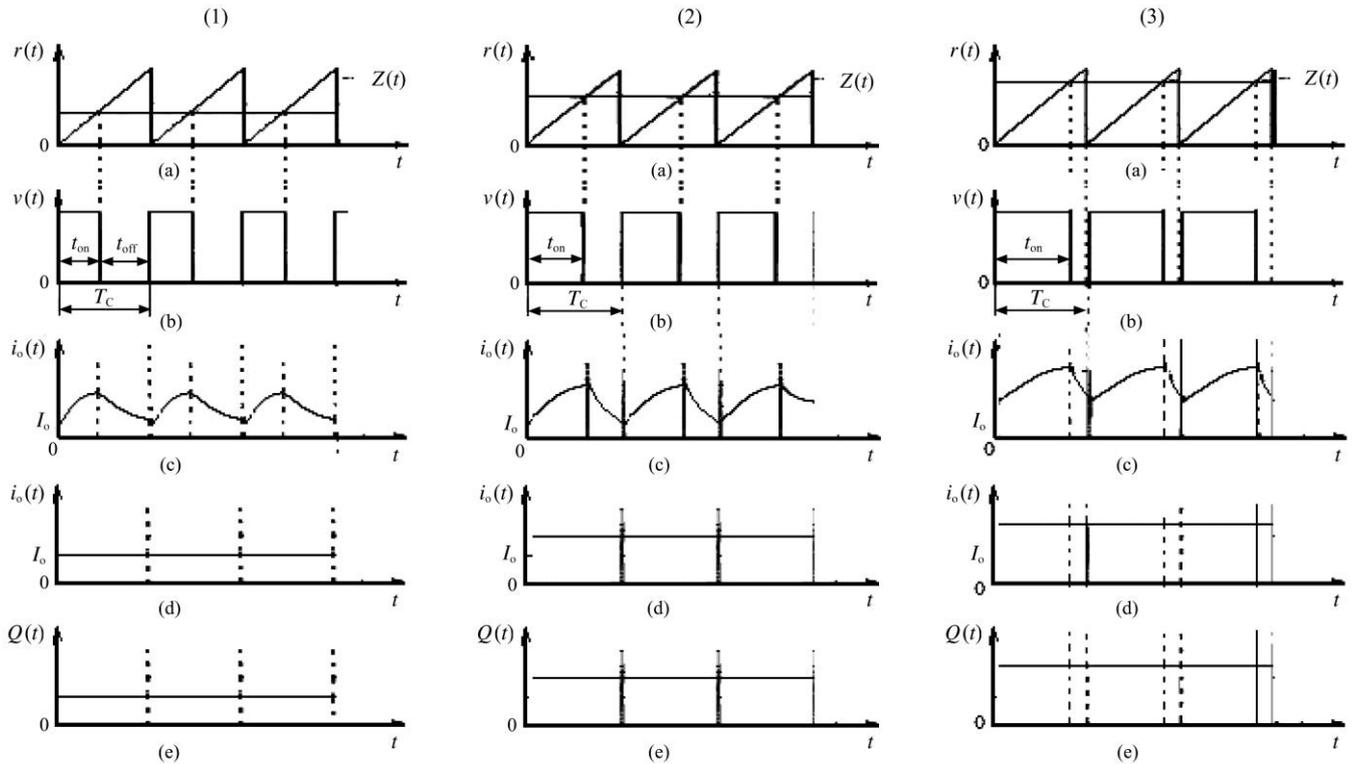
Figure 2 Wave figures of control principle for PWM continuous variable-rate spray. For duty cycles: (1)<(2)<(3).
