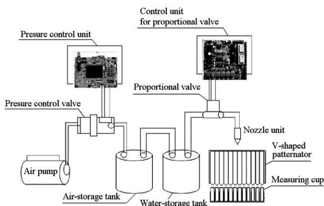
Figure 3 Experimental platform of PWM continuous variable-rate spray
