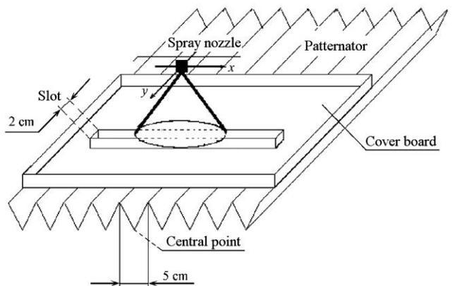
a. Schematic diagram of experimental setup for collecting data
