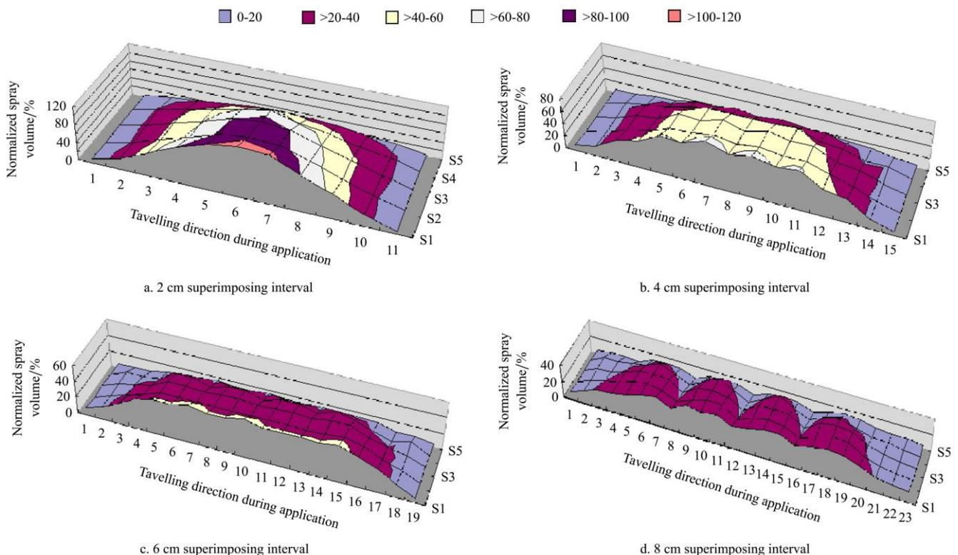
Figure 9 The 3-D spatial-temporal spray distribution pattern. S1, S2, ....., mean the span of deposit surface
