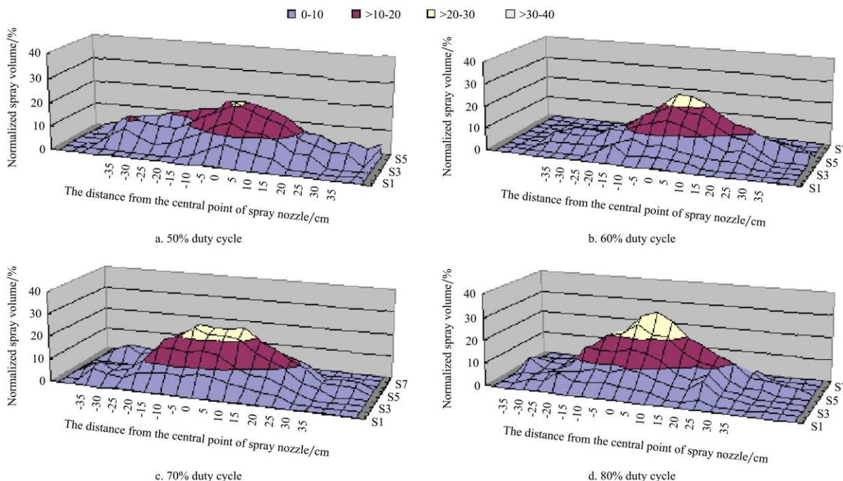
Figure 8 The 2-D spatial spray distribution pattern. S1, S2, ..., S7, mean the span of deposit surface.
