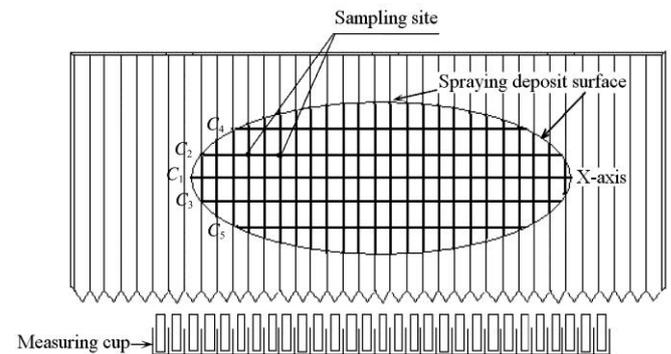
Figure 5 Schematic diagram for modeling 2-D spray distribution
