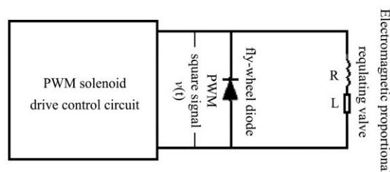
Figure 1 Schematic of control principle for PWM continuous variable-rate spray
