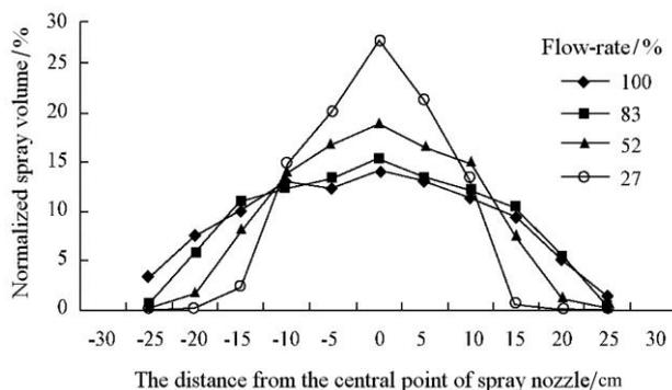
Figure 7 The 1-D spray distribution pattern
