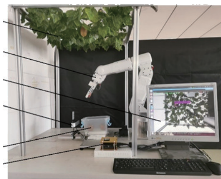
Note: 1. Indoor kiwifruits scaffolding; 2. S6H4D Plus six-axis manipulator; 3. Identification interface; 4. ZED binocular stereo camera; 5. Collection box; 6. Jetson Xavier NX system a. Indoor picking experiment
