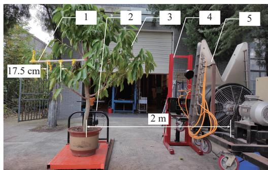
1. Sampling rod 2. Electric flat board vehicle 3. White magnolia tree 4. Double gantry manual stacker 5. Tower air-assisted spray test bench
