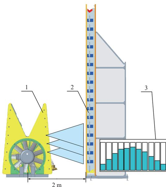
1. Tower air-assisted spray test bench 2. Lamellae vertical patternator 3. Liquid collector
