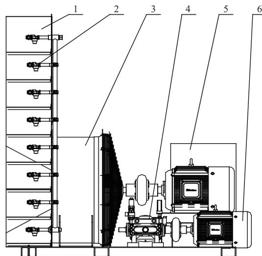
1. Tower airflow channel 2. Nozzle 3. Axial fan 4. Plunger pump 5. Control box 6. Motor
