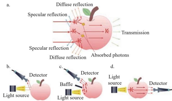
Note: Distribution of incident light in fruits (a) and different assessment modes based on specular reflection (b), diffuse reflection (c) and transmission (d)<sup>[78]</sup>.
