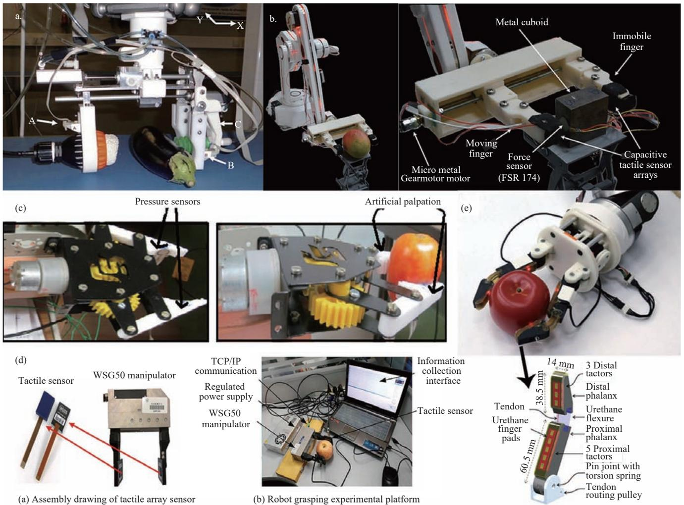
Note: a. Accelerator sensors mounted on gripper to assess the firmness of eggplant<sup>[64]</sup>; b. Capacitive tactile sensor array to assess the firmness of mango<sup>[69]</sup>; c. Piezoresistive flexible tactile sensor to classify the firmness of vegetables<sup>[65]</sup>; d. Distributed piezoresistive tactile sensor array on the two finger manipulator<sup>[66]</sup>; e. Under-actuated two-finger manipulator equipped with 8 tactile sensing units on each finger<sup>[67]</sup>.
