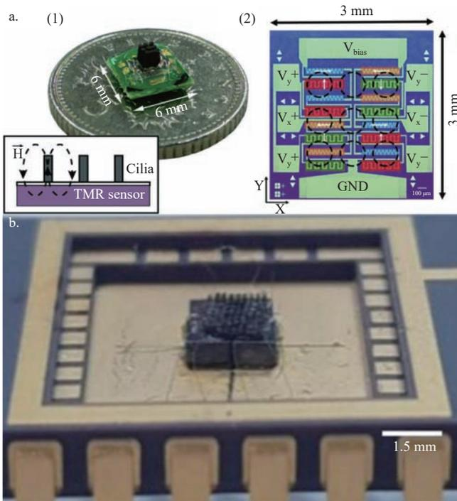
Note: a (1) Cilia sensor, with a 3×3 cilia matrix configuration; (2) Microphotograph of the sensor die<sup>[71]</sup>. b. Optical image of the device wire bonded to a chip carrier, with the giant-magnetoresistive (GMR) sensor chip integrated with 100 artificial cilia<sup>[72]</sup>.
