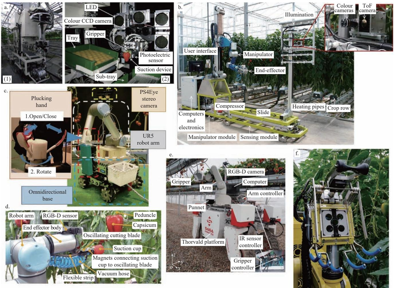
Note: a. Strawberry-harvesting robot<sup>[39]</sup>; b. Components of the sweet pepper harvesting robot<sup>[37]</sup>; c. Tomato picking robot gets color extracted from 3D colored point cloud and picking based on threshold<sup>[42]</sup>; d. Sweet pepper harvesting robot<sup>[44]</sup>; e. Strawberry harvesting robot with optimized gripper<sup>[40]</sup>; f. Sweet pepper harvesting robot with cutting device, Fotonic F80 camera, LED illumination, and fruit catching device<sup>[43]</sup>.
