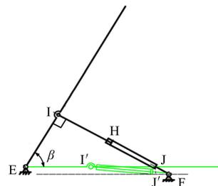
Note: E, I, and F are revolute joints, IJ is a damper spring, H is a sliding pair, J is the fixed joint of the damp spring and rod JF,  $\beta$  is the rotation angle, I'J' is the damp spring when the cover plate is horizontal.
