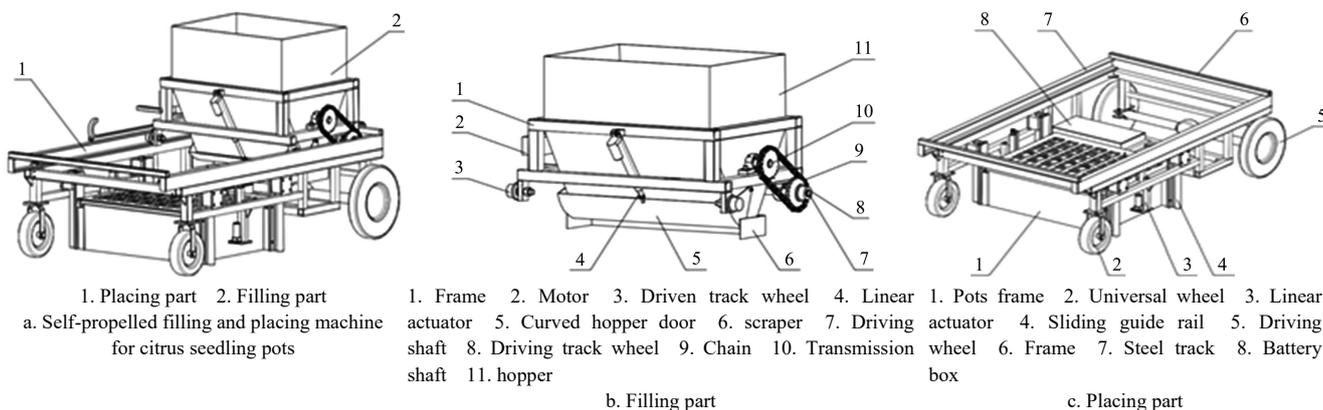
Figure 1 Structure of self-propelled filling and placing machine for citrus seedling pots
