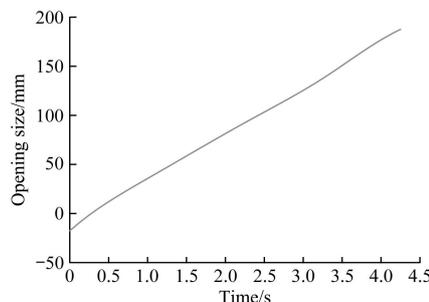
Figure 7 Diagram of the hopper door opening size and time
