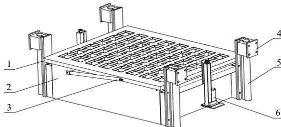
1. Pot frame cover 2. Pot frame 3. Damper spring 4. Connecting plate 5. Guide rail 6. Linear actuator
