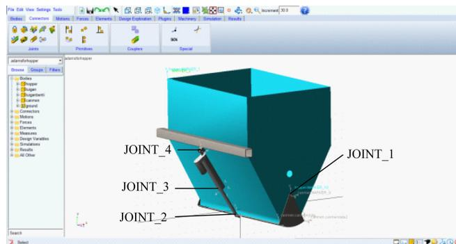
Figure 4 Hopper door mechanism in ADAMS
