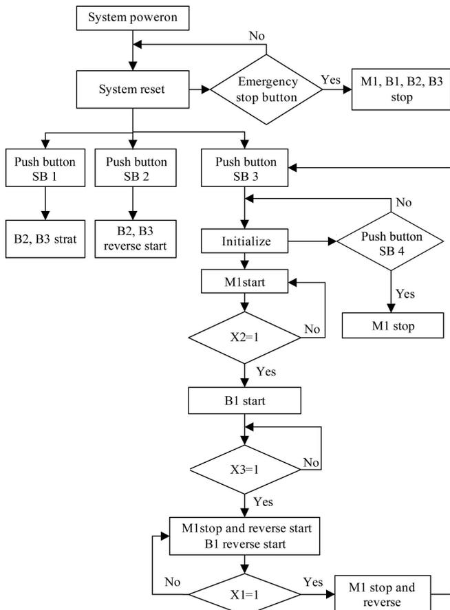
Figure 15 Control flow diagram of control system
