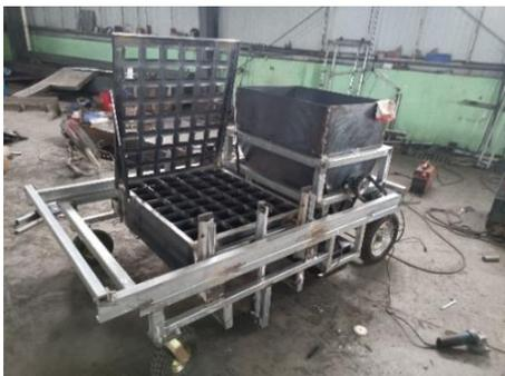
Figure 16 Prototype of the self-propelled citrus seedling pots filling and placing machine
