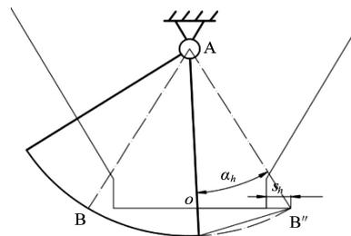
Figure 6 Diagram of hopper door opening
