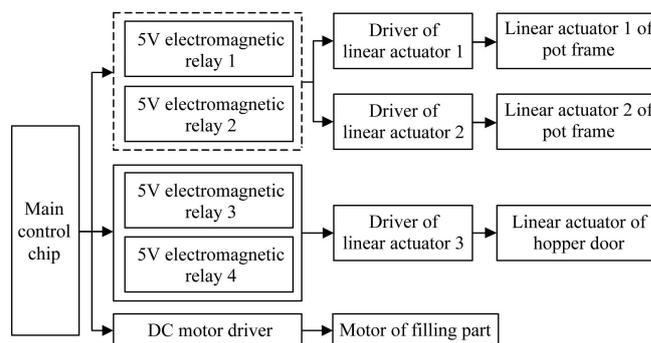
Figure 14 Hardware of control system
