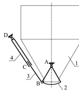
Figure 2 Hopper door mechanism
