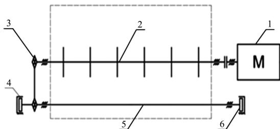
1. DC motor 2. Mixing shaft 3. Chain 4. Steel rack 5. Driving shaft 6. Driving wheel
