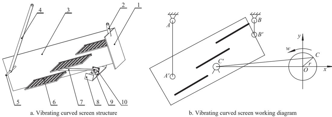
1. Horizontal baffle 2. Left boom 3. Side baffle 4. Right boom 5. Right boom support 6. Curved screen 7. Rocker 8. DC motor frame 9. Crank 10. DC motor.  $O$  point is the coordinate origin;  $x, y$  is the coordinate axis;  $L_{OC}, L_{AA'}, L_{BB'}, L_{CC}$  are the crank length, left boom length, right boom length, rocker length, mm;  $\omega$  is the crank speed, r/min;  $r$  is the eccentricity of the vibrating curved screen distance, mm.
