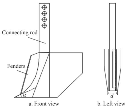
Note:  $\alpha$  is the opening angle of the furrow opener blades, and  $d$  is the width of the furrow openers.
