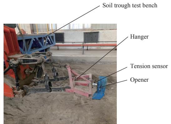
Figure 3 Ditching resistance system
