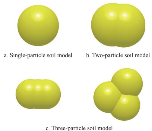
Figure 5 Soil particle model
