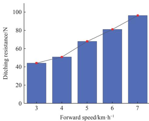
Figure 9 Relationship between the forwards speed and ditching resistance
