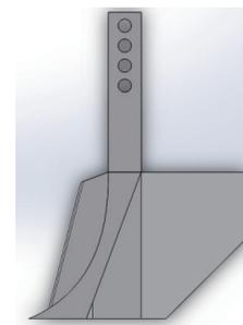
Figure 4 Simulation model of the furrow opener
