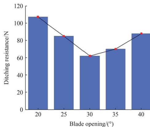
Figure 7 Relationship between the blade opening angle and ditching resistance
