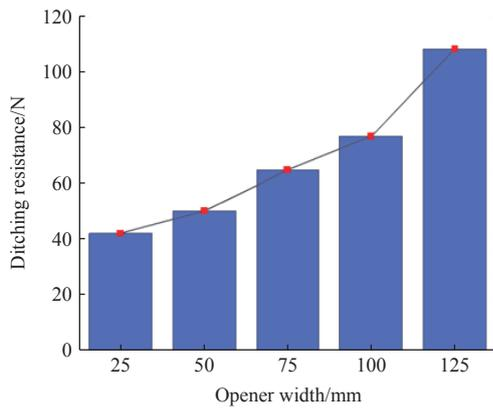
Figure 8 Relationship between the furrow opener width and ditching resistance
