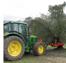
Figure 4 Mechanical trunk shaking systems
