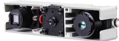
Figure 2 RGB-D camera (Orbbec Astra Mini)
