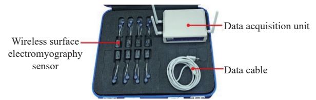
Figure 7 sEMG signal test system
