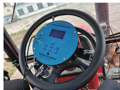
Figure 6 Torque measurement of the tractor steering wheel
