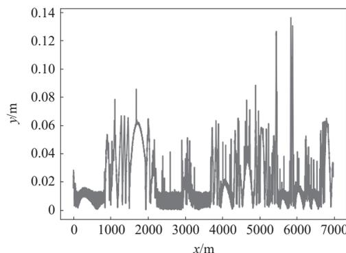
Note: y represents the lateral deviation of the farm vehicle from the reference path; x represents the distance walked by the tractor.
