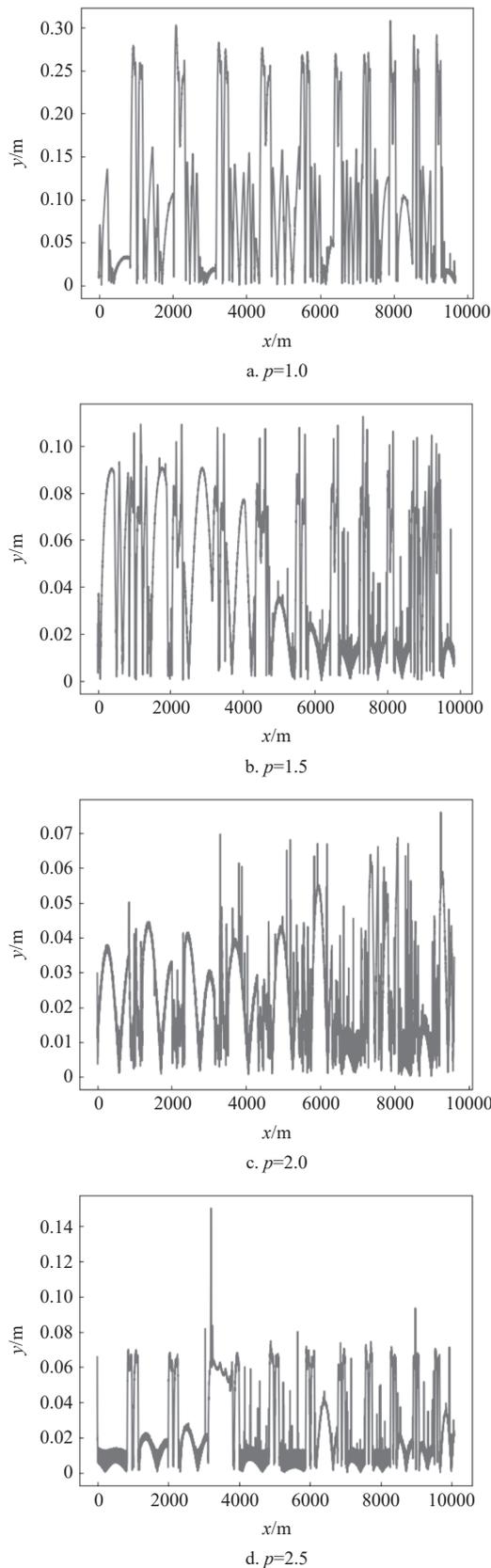
Note:  $y$  represents the lateral deviation of the farm vehicle from the reference path;  $x$  represents the distance walked by the tractor.
