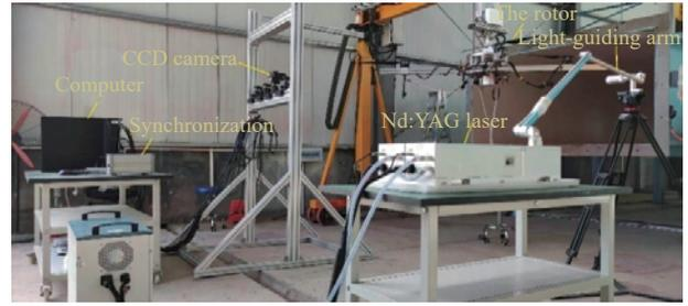
Figure 7 Particle image velocimetry (PIV) system
