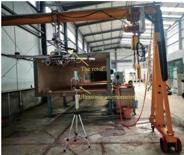
a. Two-phase-flow visualization system and ultrasonic anemometer
