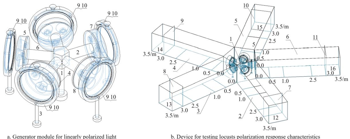
a. Generator module for linearly polarized light
