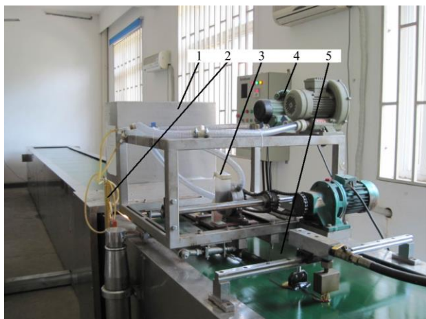
1. CCD detector 2. Manometer 3. Pneumatic precision metering device for rapeseed 4. Air fan 5. JPS-12 test stand of the precision metering device
