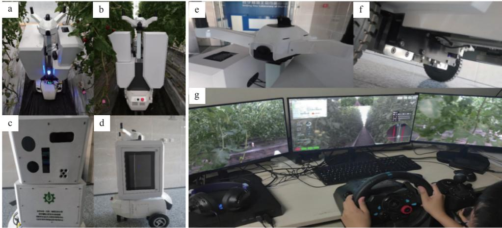
Note: a and b: The front and rear views of the robot's structure, respectively; c and d: The sensor gimbal on the left side and the control box on the right side of the robot; e: The camera and signal transmission device used for remote control; f: The bottom-mounted LiDAR sensor employed for obstacle avoidance; g: The actual workflow of remote control operations.
