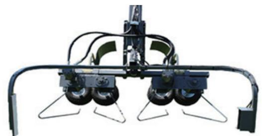
Figure 6 Extraction type detasseling device of 204SP detasseling machine<sup>[15]</sup>
