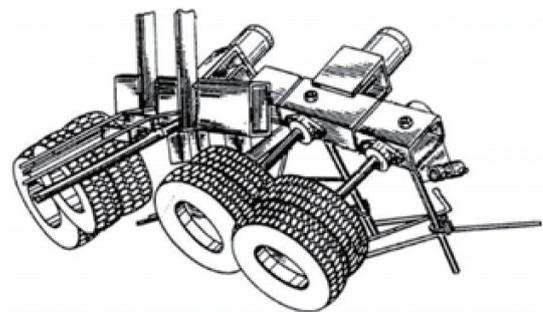
Figure 5 Inflatable-tire-extraction type detasseling device<sup>[16]</sup>
