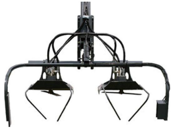
Figure 3 Cutting type detasseling device of 204SP detasseling machine<sup>[15]</sup>
