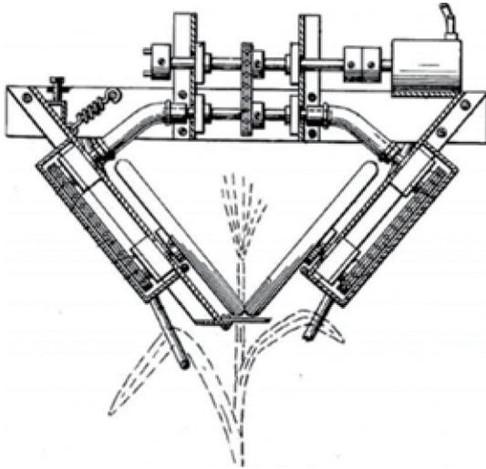
Figure 1 Clamping cutting detasseling mechanism<sup>[11]</sup>
