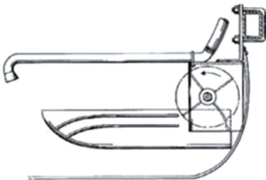
Figure 2 Air-assisted maize detasseling device<sup>[12]</sup>
