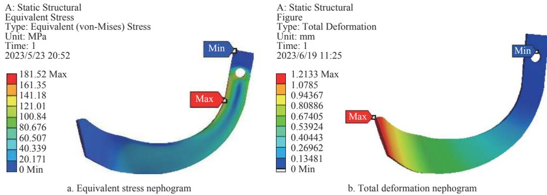
Figure 15 FEM simulation results
