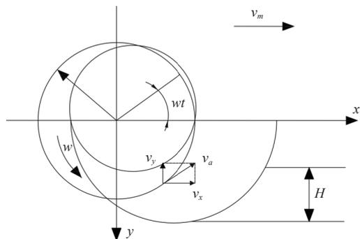
Note:  $v_m$  represents the forward speed, m/s;  $w$  represents the tool speed, rad/s;  $H$  represents the tillage depth, m;  $v_x$ ,  $v_y$ , and  $v_a$  are the horizontal and vertical separation and convergence velocities of the tool at that point, m/s.
