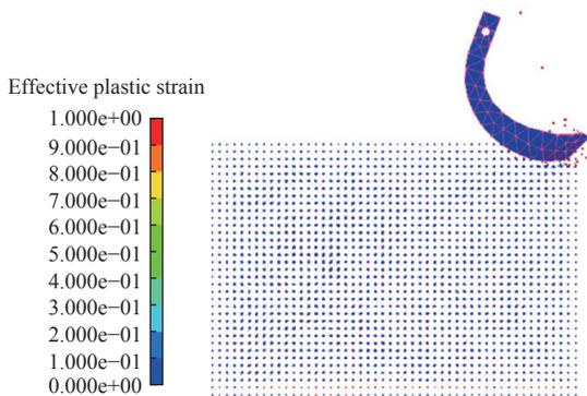
Figure 10 Stress changes during soil cutting simulation
