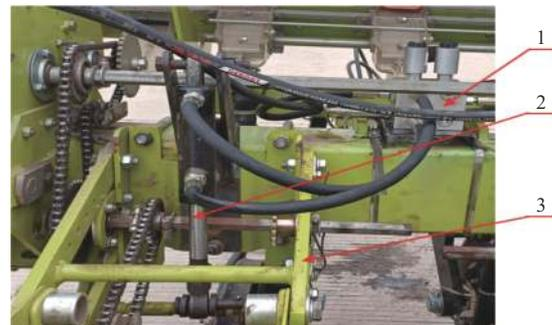
1. Proportional pressure regulator 2. Hydraulic cylinder 3. Parallel four-bar mechanism
