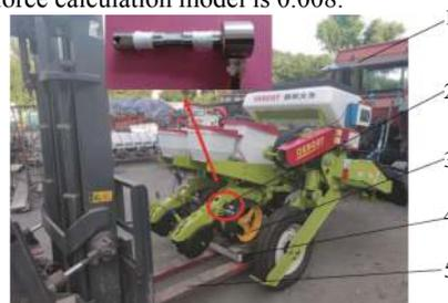
1. Tractor 2. Sensing device 3. Gauge wheels 4. Electronic scale 5. Front fork of the forklift
