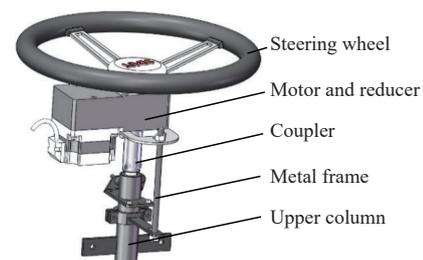
Figure 2 Installation of steering mechanism
