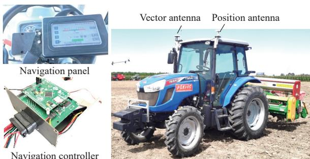
Figure 1 The wheeled tractor with the navigation system
