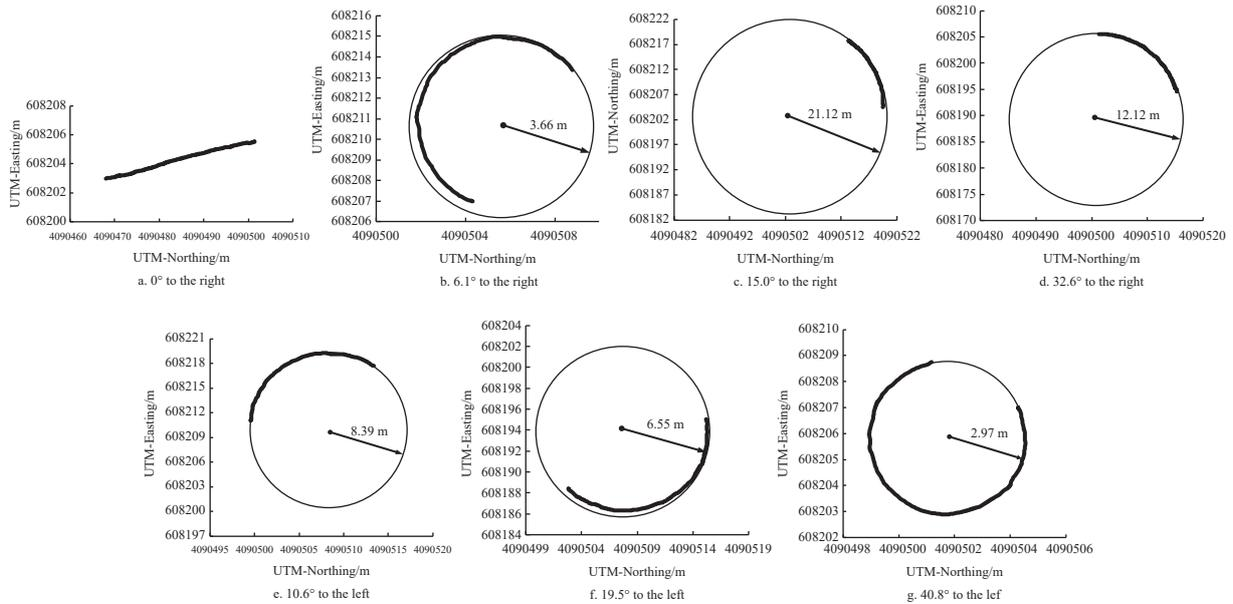
Figure 6 Turning by a target steering angle  $\varphi_d$
