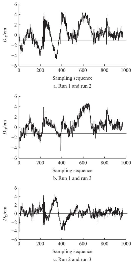
Figure 9 Variation of difference of lateral error between different runs
