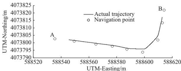
Figure 7 Autonomous navigation along the target path defined by navigation points
