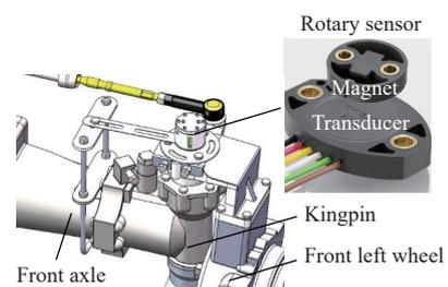
Figure 4 Installation of the rotary sensor
