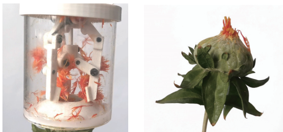
a. Filaments in process of clamping b. After the filaments clamped
