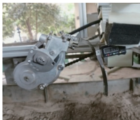
Figure 14 Measurement of the minimum distance between the transplanting arm and seedling delivery device
