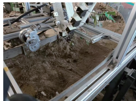
Figure 11 Test bench for sweet potato seedling
