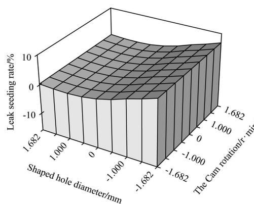
Figure 7 Interaction of shaped hole diameter and the rotating speed of cam
