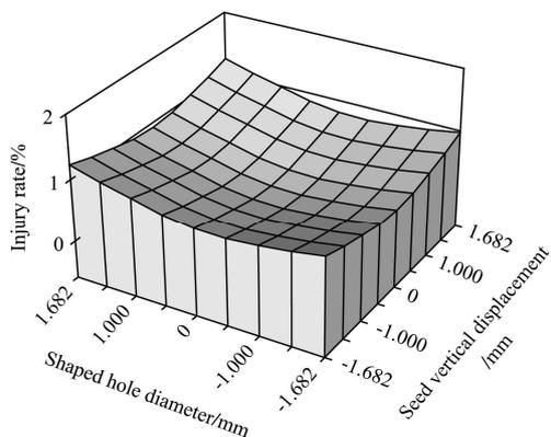
Figure 9 Interaction of shaped hole diameter and the vertical displacement of rice seeds
