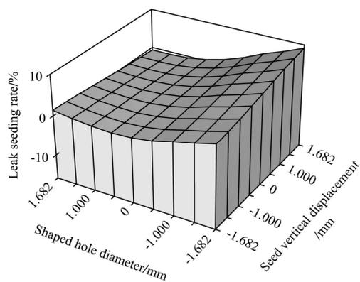
Figure 6 Interaction of shaped hole diameter and the vertical displacement of rice seeds
