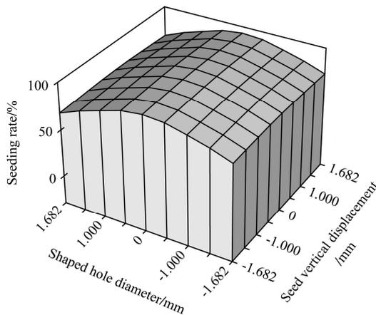
Figure 3 Interaction of shaped hole diameter and the vertical displacement of rice seeds
