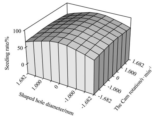
Figure 4 Interaction of shaped hole diameter and cam rotating speed
