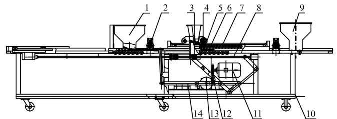
1. Subsoil box; 2. Compaction wheel; 3. Seed box; 4. Seed-brushing wheel; 5. Shaped hole plate; 6. Plate turnover; 7. Seeding raising tray; 8. Push rod of seed box; 9. Surface soil box; 10. Frame; 11. Motor; 12. Transmission chain; 13. Speed reducer; 14. Connecting rod to frame body
