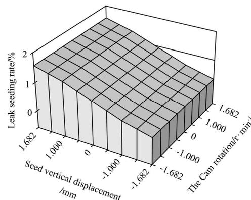
Figure 8 Interaction of the vertical displacement of rice seeds and the rotating speed of cam
