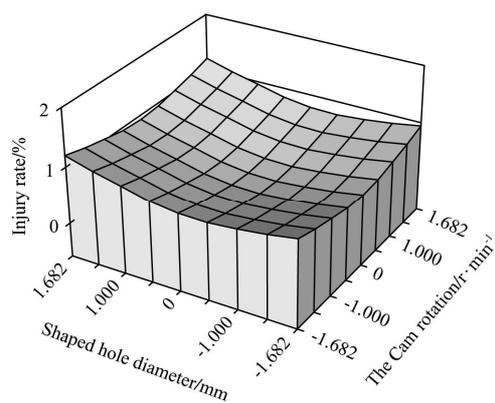
Figure 10 Interaction of shaped hole diameter and the rotating speed of cam
