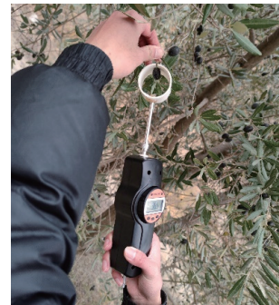
Figure 5 Measurement of fruit stem restraining force
