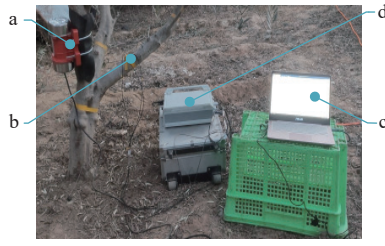
1. Vibrating motor 2. Acceleration meter 3. Computer 4. Data collector
