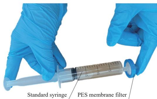
Figure 10 Obtaining soil extracts using an easily conducted extraction filter (ECET)
