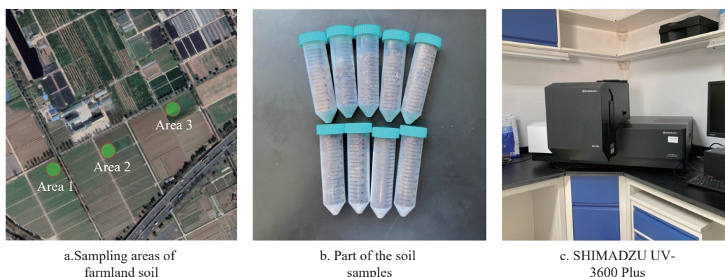
Figure 11 Application test setup for the portable soil nitrate-nitrogen determination device
