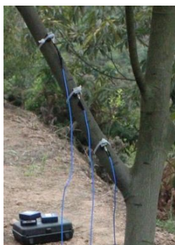
Figure 3 Photography of the sensors mounted on the tree
