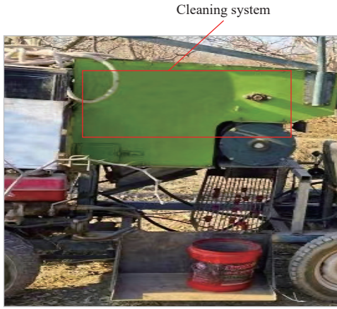
Figure 3 Physical drawing of cleaning system
