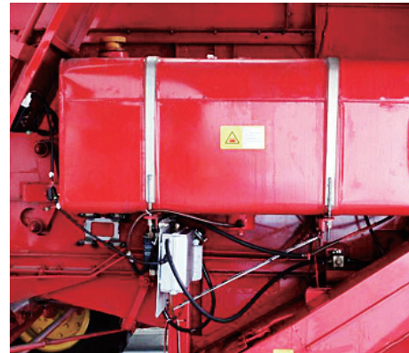
Figure 4 Installation diagram of real-time fuel consumption monitoring
