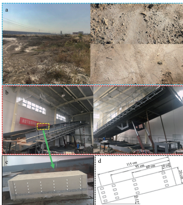
Note: a. site pictures of borrow area; b. experimental apparatus (runoff erosion trough and rainfall simulator); c. experimental soil flume; d. sampling point diagram.
