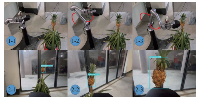
Figure 18 Demonstration of pineapple picking process in robot system
