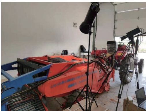
Figure 16 Bench test and high-speed photography layout plan
